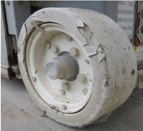
Excessive damage to sidewall and separation between tyre and rim
